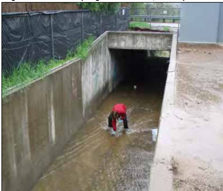
Figure 9-6. Grab Sampling at Mid-Stream, Mid-Depth
