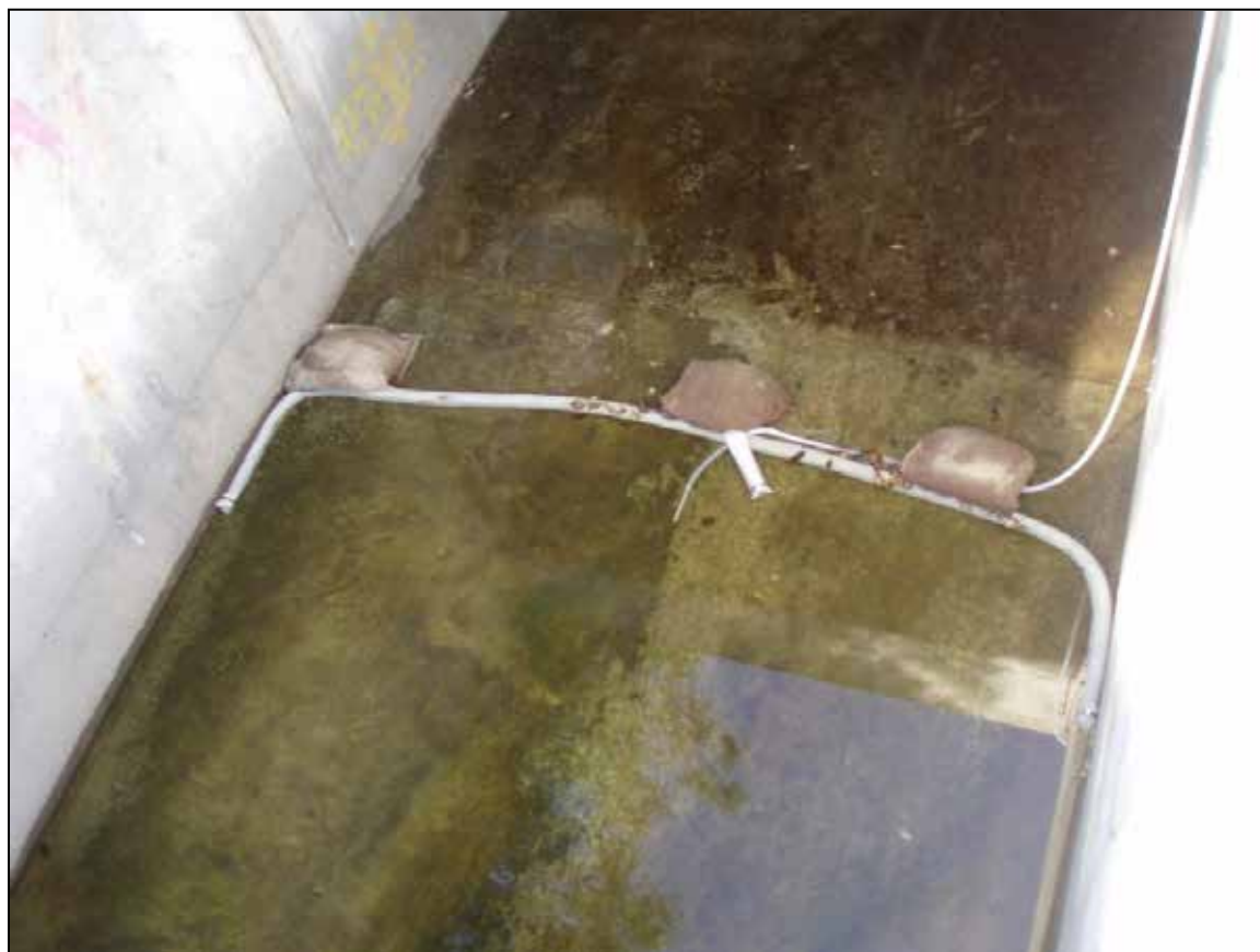
Figure 9-8. Typical Wet-Season, Dry-Weather Sampling Configuration
