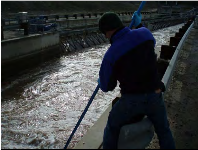
Figure 9-7. Grab Sampling Using Extended-Reach Swing Sampler
